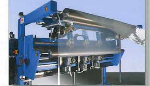
Vertical edge trimming and multiple longitudinal cut
