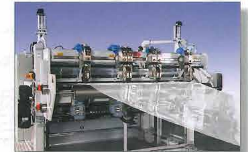
Horizontal edge trimming and multiple longitudinal cut
