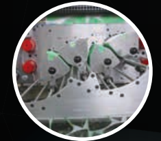
Labels for beer bottle necks, 150 x 140 mm – 4 cavities, aluminium 12 micron, perforated and embossed 110 micron
